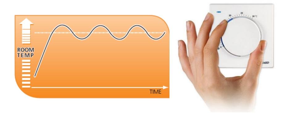
With conventional on/off controls, why even fit a condensing boiler.....No intelligence
